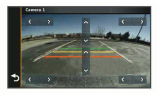
5 Use the arrows in the center of the screen to move the colored distance guidance lines up or down.
